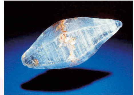
Corundum is the base material of In-Ceram; here: sapphire variety
